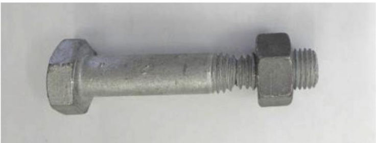
(c) M20 HR specimen after test
